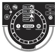
When the field service access door is open, the user has access to the RESET (5) DISABLE , Fire Test , AutoLearn and Instant Fault Finder functions. When the Instant Fault Finder function is activated, the Smoke Dial converts to a fault indicator, with the dial segment numbers corresponding to the faults listed below.
